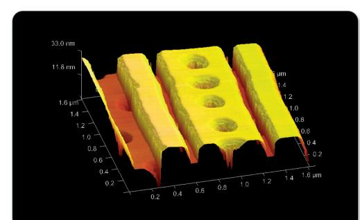
Closed-loop topography map of a kerf test structure showing contact holes inside dual-damascene trenches. The combination of the Dimension scanner and a Bruker FIB probe enabled mapping of this challenging geometry without damage to the probe tip.
