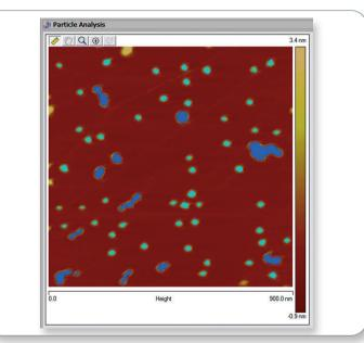
A complete set of processing and analysis functions is embedded in the system's architecture. A single mouse click transfers images from real-time to analysis without interrupting ongoing data acquisition. Here, a particle analysis is performed on silver nanoparticles, which are potent and broad-spectrum antimicrobial agents. Image size 900nm. Sample courtesy of Dr. Perry, School of Medicine, Loma Linda University, CA.
