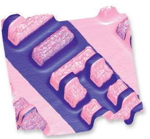
Accurate 2D dopant profiling on SRAM sample using Dark Lift SCM. Image size 15µm.
