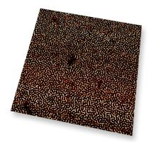
Closed-loop phase image revealing the micro-phase separation in a poly(styrene-bbutadiene-b-styrene) triblock copolymer. Image size of 2µm.
