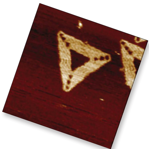
Individual triangular self-assemblies of origami-DNA on mica imaged in liquid reveal individual strands and fine structure at the connection points. 250 nm closed-loop image. (Sample courtesy of P. Rothemund, Caltech.)
