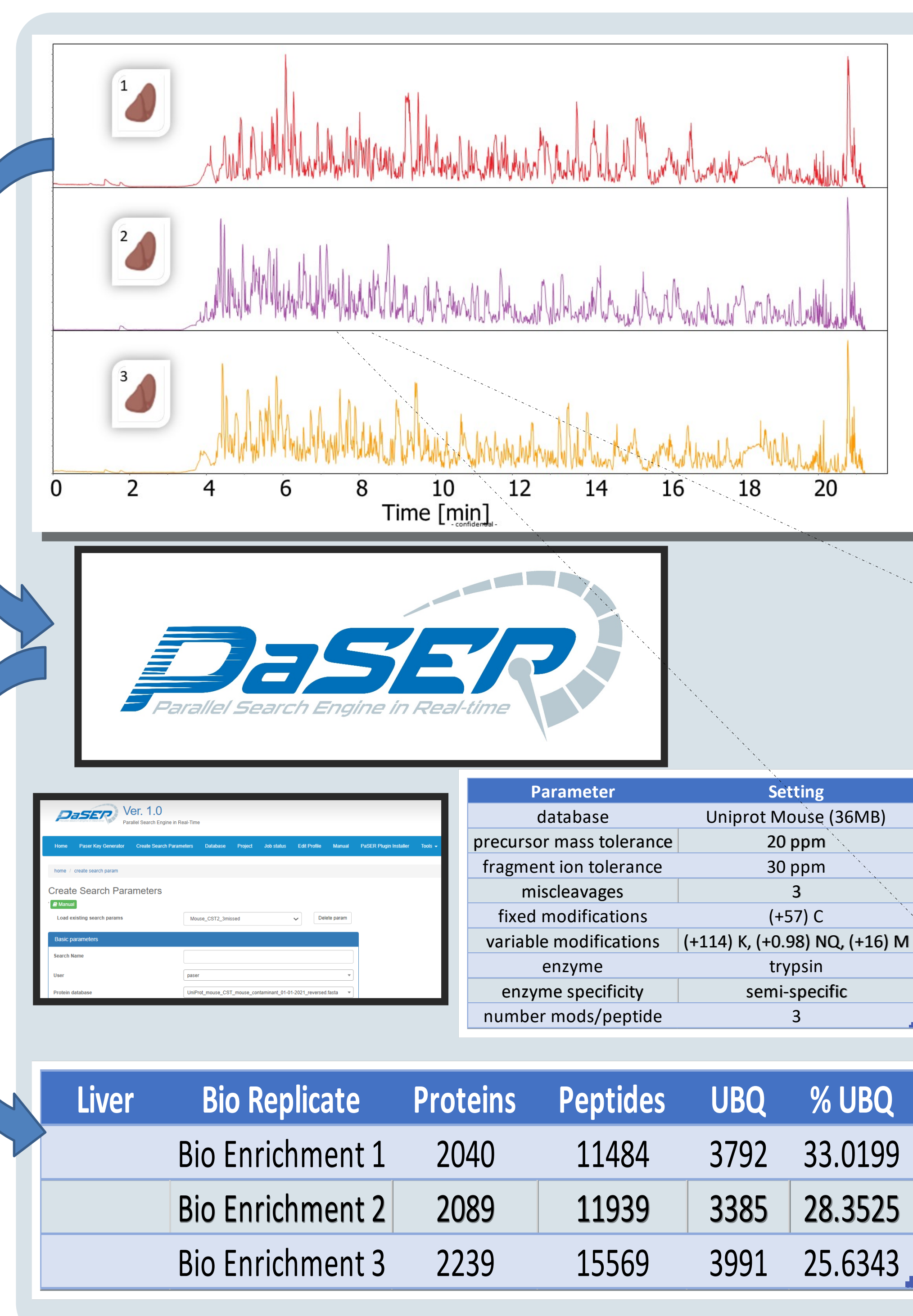
Figure 2: PaSER real-time ID of 50 samples per day Ubq enriched mouse liver: 21 minute Base-peak chromatograms of 3 biological replicates of Ubq enriched mouse liver. Real-time database searches are performed by PaSER with non-specific enzyme settings and multiple variable modifications. Deep proteome coverage and high enrichment efficiency using CST Ubq-scan kit.
