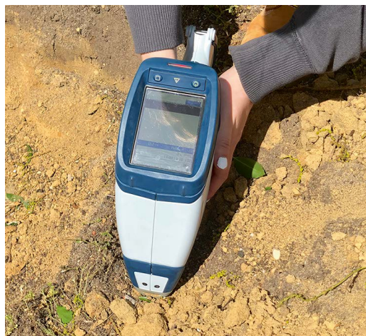
Soil analysis with the S1 TITAN
