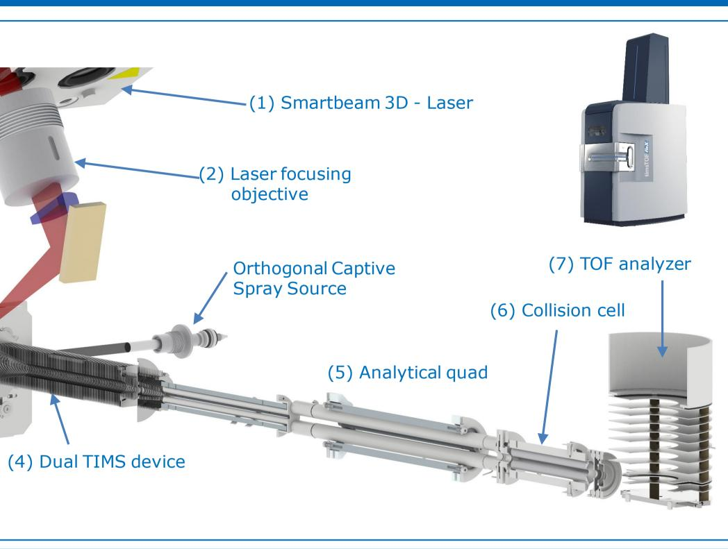
**Fig. 1: Ion optical components** of the timsTOF fleX, a dual ion source trapped ion mobility separation quadrupole orthogonal time of flight instrument
