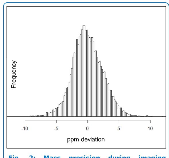
Fig. 2: Mass precision during imaging performance without lock mass. Histogram plotting the mass drift for the peak m/z556.23 over six consecutive measurements of rat brain sections. In total,  $\sim 2.2$ million pixels with a lateral resolution of 20 um pitch size were acquired; the acquisition of all six sections was approximately 30 hours.
