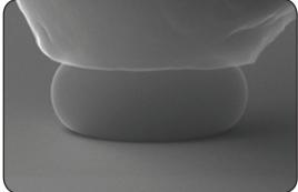
Silica particle compression with 1 mN DC, 100  $\mu$ N at 10 Hz AC load. Particles shown exhibit viscoplastic creep under load.
