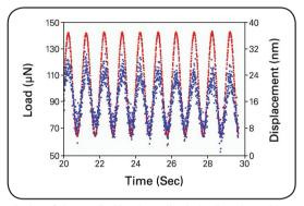
A plot of the applied load amplitude (red) and resulting displacement (blue) data from a 1 Hz dynamic loading test on a metallic thin film.
