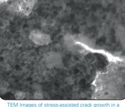
IEM Images of stress-assisted crack growth in a metallic thin film subjected to a tensile fatigue stress. Note the void formation leading to crack initiation (stage I fatigue, top image) followed by crack growth (stage II fatigue, bottom image).
