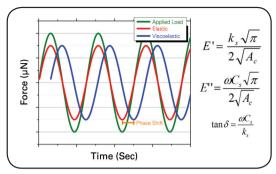
Schematic of sinusoidal force and resultant displacement data as measured using nanoDynamic Mode. Equations for storage (E') and loss (E'') modulus are given on the right.
