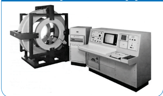
1983: One of the first whole body MRI tomographs with air coil magnet.
