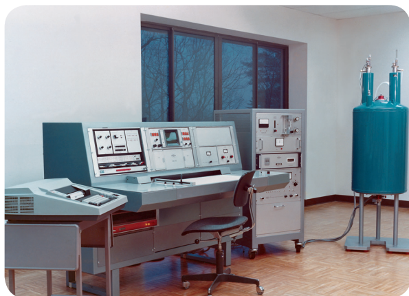
1972: WH270, Bruker's first high-field NMR spectrometer based on superconducting magnet technology.
