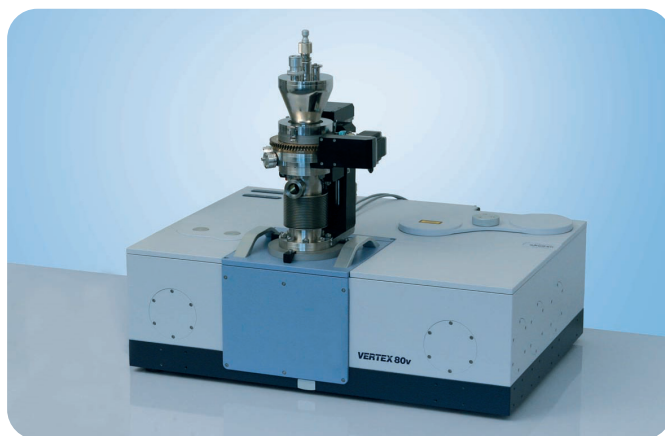
Fig. 5: VERTEX80v vacuum FTIR spectrometer with automated liquid N 2 or He flow through cryostat for up to 6 samples.
