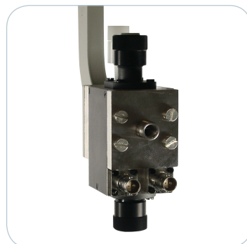
Dual Mode resonator for detection of forbidden transitions for S > 1/2
