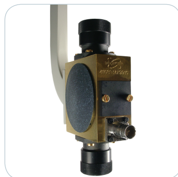
TM mode resonator for large aqueous volumes
