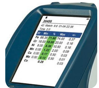
Bruker S1 TITAN handheld XRF screen showing 2 second results of 304SS identification test
