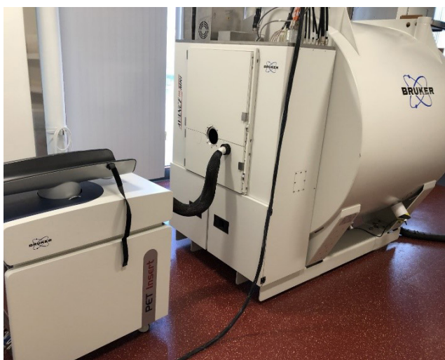
Figure 1. Top: PET Insert sitting on support cart with all PET electronics. Bottom PET Insert being used inside the magnet bore of the Biospec 4.7 T.
