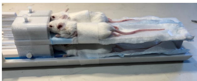
Figure 2 Custom designed 4 mouse bed (top) at Martinos Center for Biomedical Imaging, MGH. Top: bed without subjects on it to show the animal housing space and nose cone and tooth bar. Bottom: animal loaded with 4 mice prior an in vivo PET/MRI imaging session.
