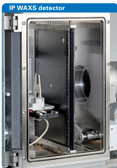
Figure 4: Close view into the extended sample chamber of the NANOSTAR showing standard sample holder and central part of the IP.
