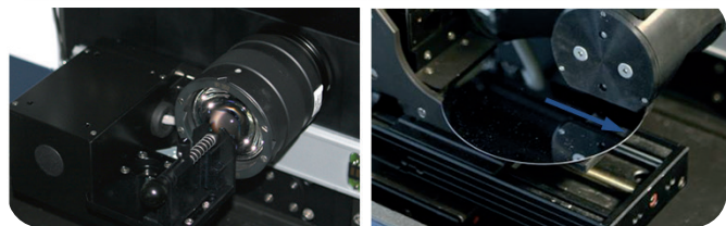
Fig. 1: Top: P.L.I.I. module adapted to INVENIO R research FTIR spectrometer. Lower left hand side: standard glass objective with vertical sample mount. Lower right hand side: mirror objective and X-Y mapping stage for convenient horizontal sample positioning.
