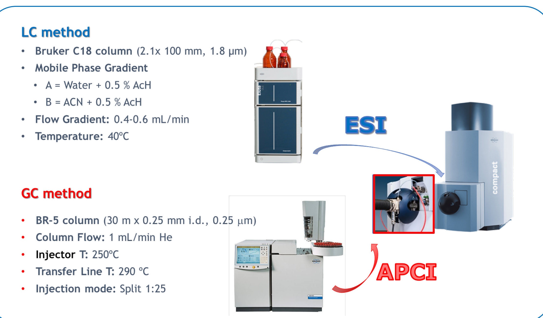
Fig. 2: LC and GC methods to analyze the olive oil extracts
